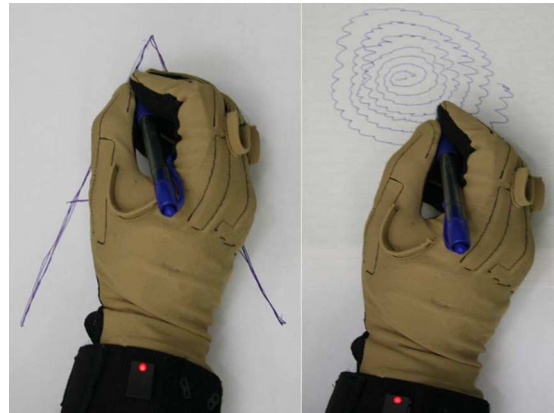
Fig. 2. Two tasks of subject 2 wearing CyberGlove: writing letter A (left) and drawing Archimedes spiral (right). Tremor is witnessed while drawing the spiral.
