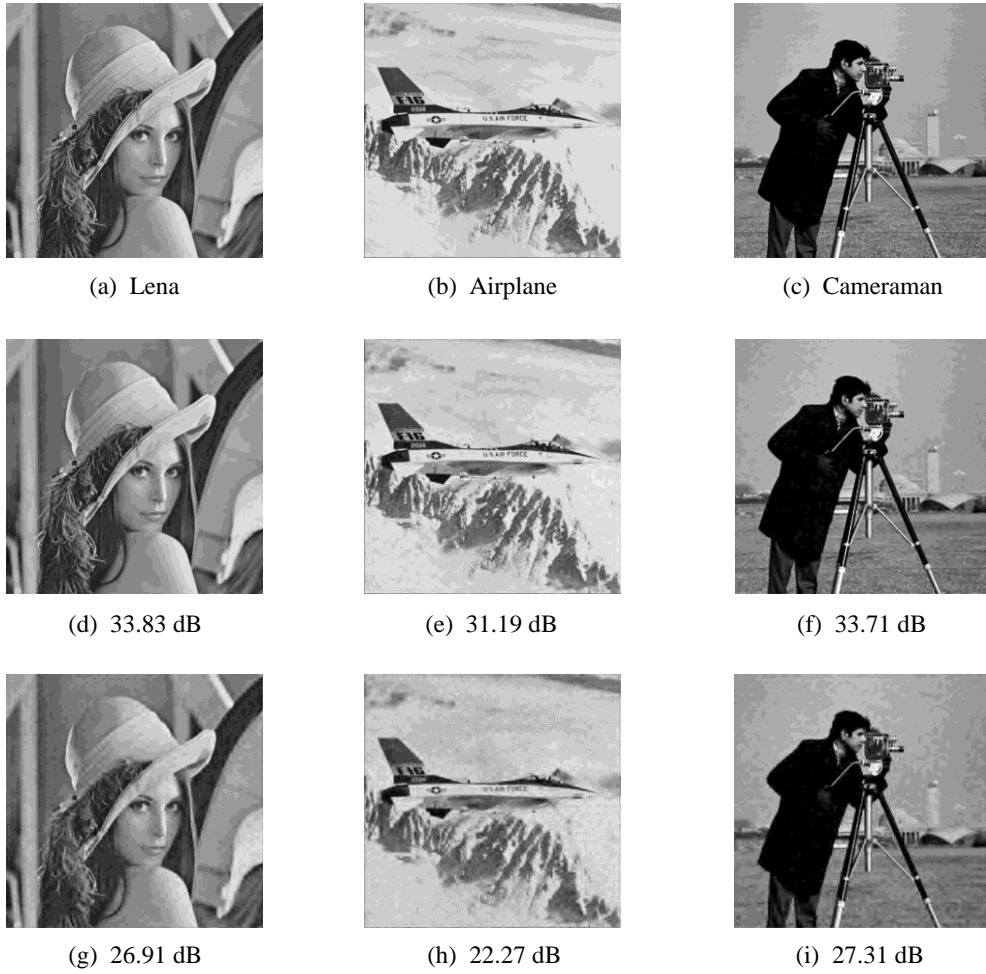
Figure 3.4.8: The original grayscale images of size 512 \times 512 are shown in the first row. The images recovered by ADM-MIQP are shown in the second row. The images recovered by MDAL are shown in the third row. Then, the PSNR value of each recovered image is averaged 10 trials at m = \lfloor 0.15n \rfloor and k = \lfloor 0.05n \rfloor
