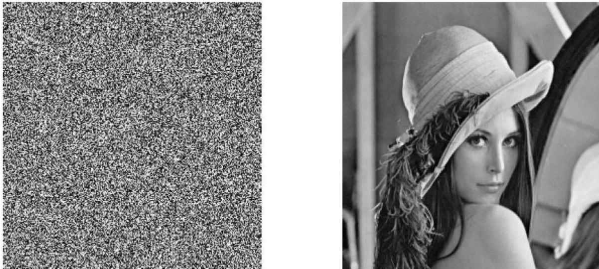
Figure 14: Comparison of a random image (independent pixels obeying a uniform distribution over [0; 255] , on the left) and the photograph of a natural scene (portrait of Lena, on the right).
