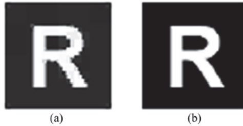
Fig. 9. Images (64 × 64 pixels) reconstructed using the best K -term Haar wavelet approximation: (a) K = 400 and (b) K = 675 [1].
