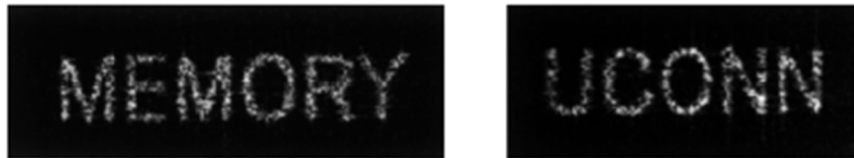
Fig. 8. Images that have been digitally reconstructed with the digital hologram of both the encrypted data and the Fourier phase mask.
