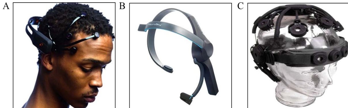
Figure 7 (A) EPOC system (Emotiv Corporation), (B) Mindset (Neurosky company), and (C) DSI 10/20 (Quasar Company).
