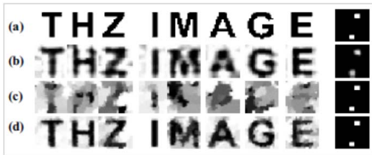
FIG. 3. Simulated results demonstrating the universality of the proposed mask. (a) Original image and reconstructed images using (b) 40 optimized masks, (c) 40 random masks, and (d) 120 random masks.
