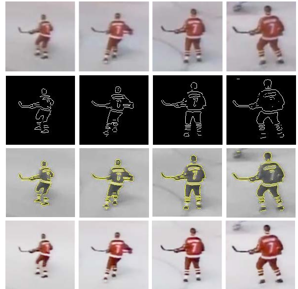
Fig 2. Image of enhancement process. From top to bottom: a) original images of hockey player. b) detection of edge c) overlapping edge on original image d) high resolution image after enhancement step. The color of object and background was modified using Sparse representation algorithm.
