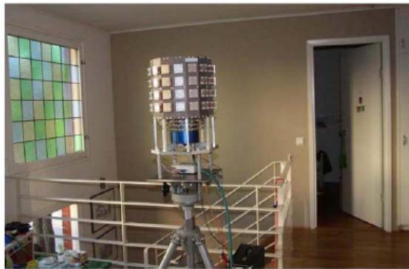
Figure 4. Massive MIMO antenna used in measurements
