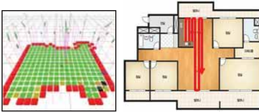
Fig. 3. SLAM and well-aligned cleaning robot path.
