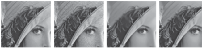
Fig. 2. Comparison with the NL-means method and proposed algorithm. From left to right: original image, noisy image ( \sigma = 10 ), the result of NL-means (PSNR 35.41) and our result (PSNR 35.20).
