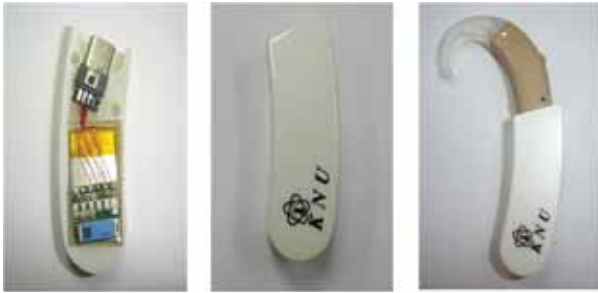
Fig. 3. Implemented Bluetooth adaptor for wireless communication.
