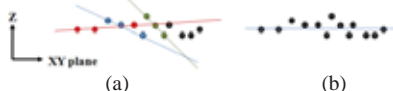
Fig 1: Model estimation of a plane using (a) three points and (b) multiple points by least square fitting
