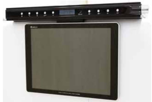
Figure 3. The implemented prototype portable kitchen TV.
