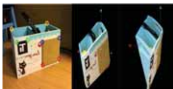
Figure 3. Verification of modeling accuracy. Target points for distance measurement(left). A virtual object at the current camera viewpoint and virtual viewpoint(middle and right).
