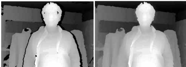
(a) Original depth image (b) Hole filling result Fig. 4. Depth image hole filling result using object segmentation
