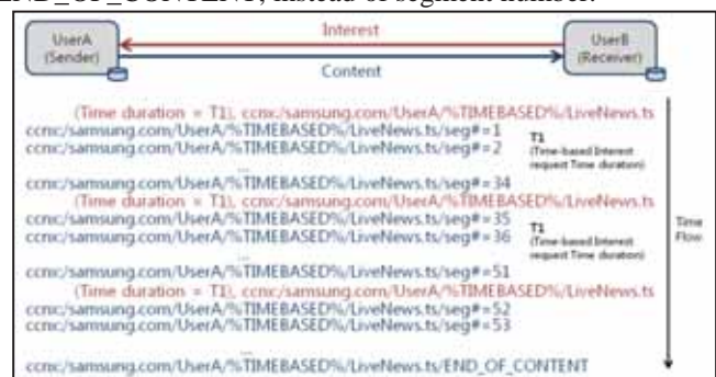
Fig. 1 Time-based Interest protocol Interest/Content segment exchange flow
