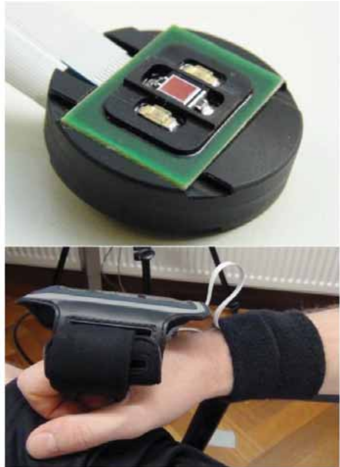
Figure 1: The optical sensor (above) and the accelerometer (below) with the connection to the optical sensor mounted on the wrist.
