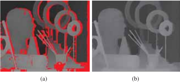
Fig. 2. Disparity fitting (a) Non-red regions are high-confidence disparities and the red region is the low-confidence region. (b) Output of the disparity fitting algorithm.
