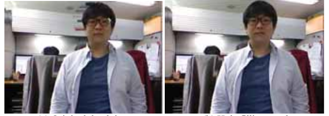
(a) Original depth image (b) Hole filling result Fig. 5. Depth image hole filling result using object segmentation
