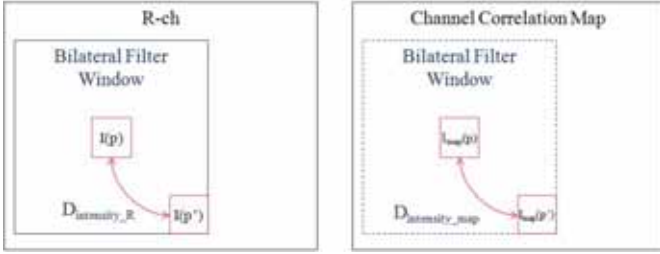
Fig. 4. Proposed bilateral filter on R channel denoising with cross-channel correlation map.
