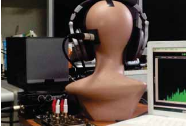
Fig. 2. Experimental setup of the FBANC based earmuffs system.
