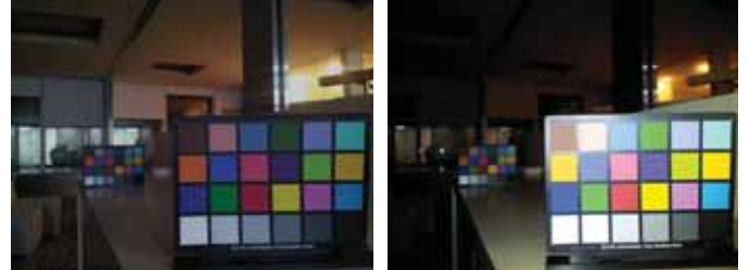
Fig. 1. Input image pair. (Left) Long exposure time without flash. (Right) Short exposure time with flash. The center is overexposed and the background becomes too dark. There are more noise in the left image.
