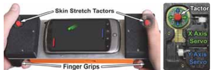
Fig. 1. Bi-manual skin stretch peripheral provides skin stretch feedback while allowing thumb-based input [left]. Internal actuation mechanism of a single skin stretch display [right].
