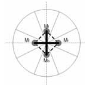
Fig. 2. 4-channel microphone array structure for front, back, left, and right microphones
