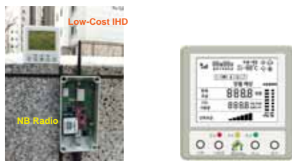
Fig. 2. 424 GHz NB radio in the area IHD server site and the IHD device for the low-cost IHD system.
