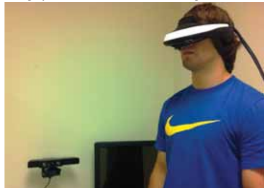
Fig. 1. The head-mounted display and tracking system are shown. The tracking system is on the left, and the user faces it in normal operation.
