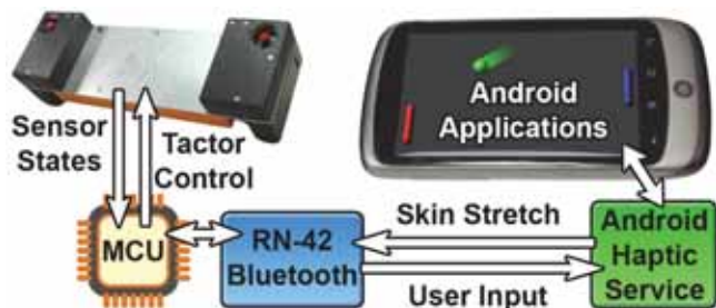
Fig. 2. Schematic of peripheral's hardware and software components.
