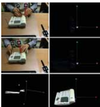
Figure 2. 3D modeling process with the brush control pen. The results of modeling the receiver of a telephone (first row), modeling the body of the telephone (second row), and the results of modeling with the brush control pen (third row).
