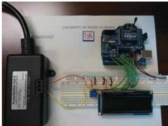
Fig. 2. Experimental node design. This prototype was built to implement the wireless-network, power-monitoring, and power-shutoff features as a proof of concept.
