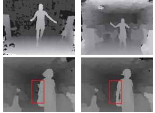
Fig. 2. Disparity results of Kinect, proposed system (upper); comparison of AD-Census [6] and proposed (lower)
