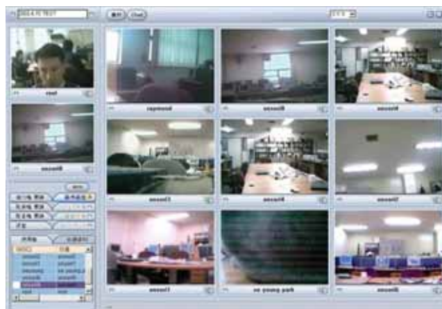
Fig. 3. In case the number of participants is increased to 6, constantly suggested voice or video transfer algorithm is applied, participants of video conference is 6, and the number of frame is 10-14, then the transfer speed is kept to 140ms. But the number of frame should be kept below 15.
