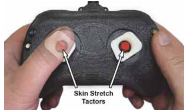
Fig. 1. Skin stretch feedback is integrated into the tops of the thumb joysticks.
