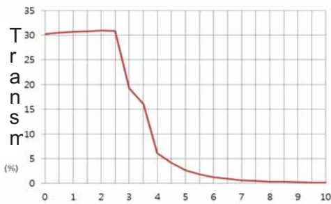
Fig.2 The light transmittance with the applied voltage of the flexible liquid crystal lens fabricated on PC substrate.
