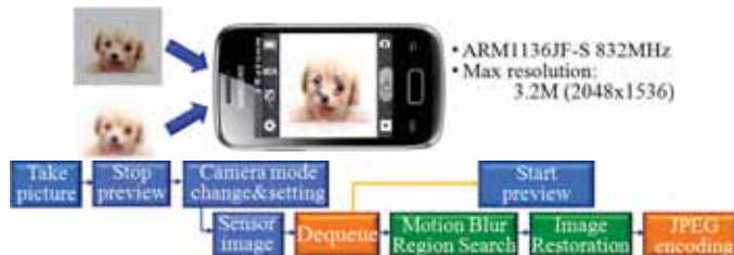
Fig. 5. Modified flow of Android camera's image capture flow
