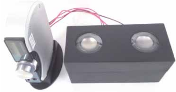
Fig. 6. Hapticon playback toolkit, which consist of a digital amplifier (left) and a pair of vibrotactile actuators (right)
