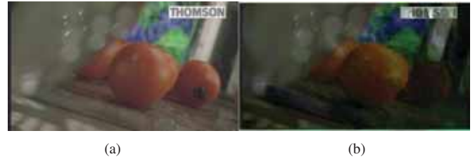
Fig. 1. Thumbnail image of HD ( 1920 \times 1080 ) sequence. (a) Full decoding method. (b) Kim's method in the transform domain [2].
