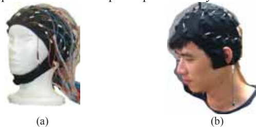
Fig.1 EEG Hats (a) traditional design (separate outputs for each channel) (b) the novel design presented in this paper (one output)
