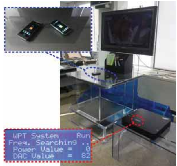
Fig. 5. Application of WPT system to simultaneous mid-power delivery for 46-inch wall-hanging LED TV and low-power battery charging for two smart phones. [Insets: Two smart phones are in charging (top); and the user interface of adaptive tracking system (bottom)]
