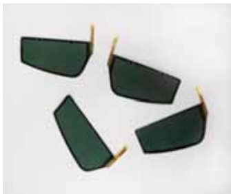
Fig. 4 The flexible liquid crystal lens fabricated in this works.
