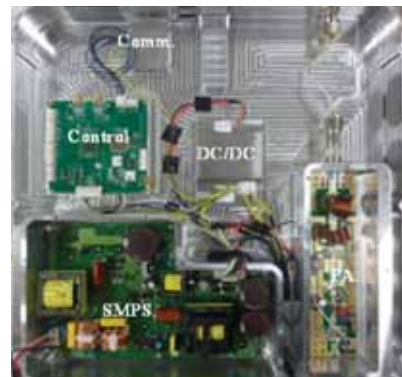
Fig. 2. Adaptive TX system; Block diagram (top) and fabricated module assembly (bottom).
