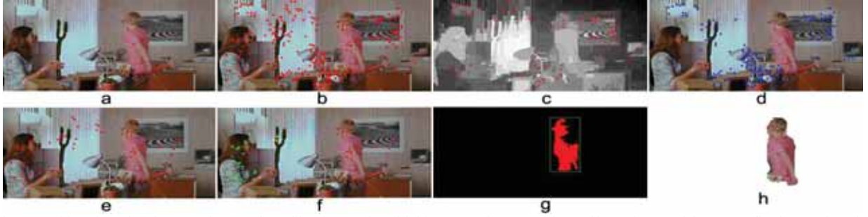
Figure 1. Object detection framework. (a) Selected keyframe; (b) Initial interest points; (c) Subset of keypoints used for camera/background motion estimation; (d) Estimated camera / background movement; (e) Outlier interest points; (f) Motion classes; (g) Saliient regions; (h) Segmented object.
