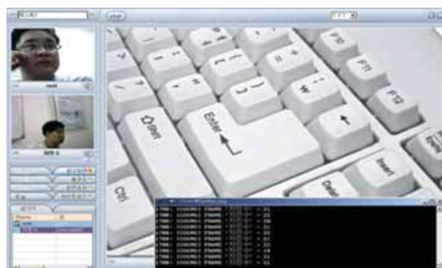
Fig.4. Not only video transfer algorithm but also channel management algorithm is applied together, and improve the rate of compression, it is transferred safely as maintaining average over than 20 frames and 30ms. As a result, the transfer speed is improved 4 to 5 times, and it showed high resolution.
