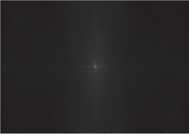
Fig. 6. 2D cross correlation function of the two consequent frames with Sobel pre-filtering.
