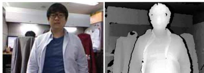
(a) Original RGB image (b) Original depth image Fig. 1. Original color(RGB) image and depth image acquired by Kinect
